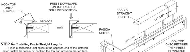
Place a concealed joint splice in the opposite end of the installed miter. Install the fascia by hooking the top and pressing the top face downward to snap fascia into place. <u>Allow a 1/4" gap between</u> <u>fascia sections for thermal expansion</u>. Review lengths of all straight pieces prior to cutting to avoid creating relatively short sections of fascia adjacent to full length sections. (DO NOT HOOK THE BOTTOM OF THE SPLICE ONTO THE RETAINER) Note: There must be a splice at every joint.
