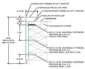
PRE-DRILL WITH 3/16-IN. DRILL BIT FOR MASONRY CONDITIONS. CONTACT US FOR APPROPRIATE RECOMMENDATIONS NEEDED TO MEET/EXCEED
