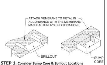
Locate sump cores where downspouts will be located. Sumps are installed prior to the retainer. The retainer butts up to side(s) of sump core. Spillouts are installed along with the fascia lengths as required. Refer to "Sump Core & Spillout Install Guide" for more info on installation if necessary.
